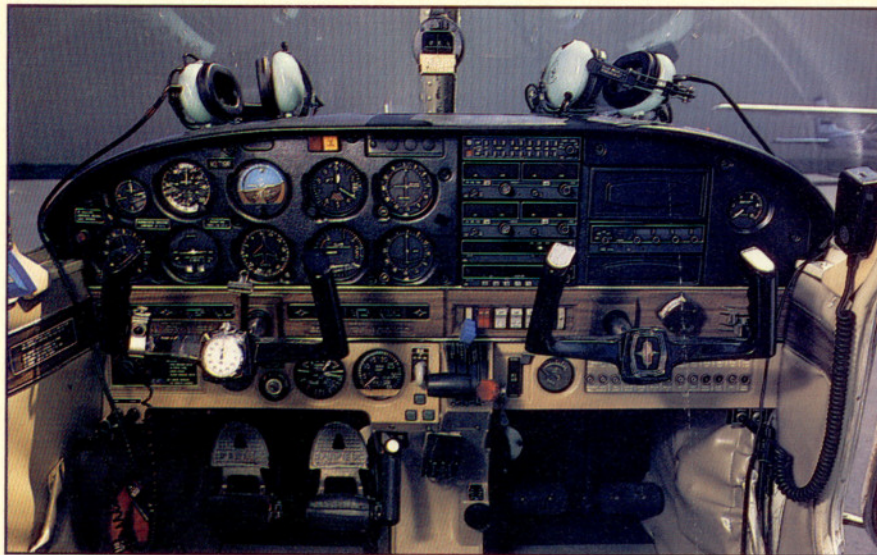
The Arrow's all-new panel featured a multi-engine-style engine power console, flight instruments arranged in a T-pattern, an avionics stack in the center and rocker switches.
